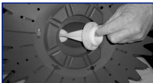
Remove from body by pulling through bottom of APC
